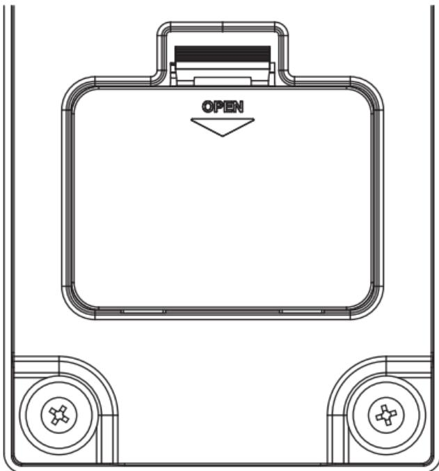
Battery compartment cover on underside of pedal snaps open and shut easily; compartment houses single 9-volt battery that lifts out easily for replacement.
