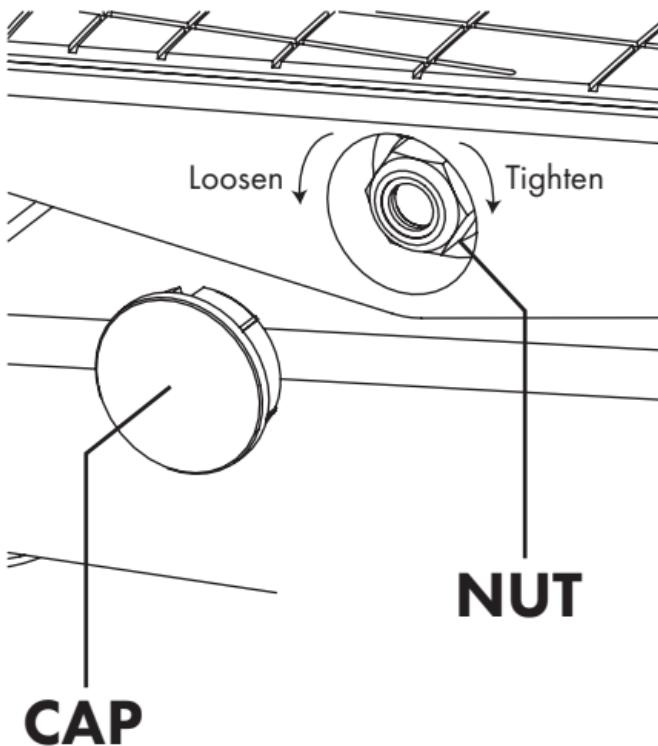
To loosen or tighten rocker movement of pedal, pry cap from right side of pedal with a small flat-head screwdriver; use 10mm socket wrench to adjust nut to pedal motion preference. To avoid damage to pedal assembly, do not over-tighten.
