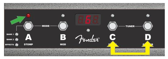
To activate the footswitch tuning function, step on buttons "C" and "D" simultaneously (double yellow arrow). In the example above, a "G" note is displayed as being particularly flat, as indicated by the illumination of the red LED above button "A" (green arrow).
