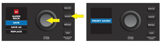
**SAVE AS:** Enables saving a preset in a different position, with or without a different name. To do this, press the SAVE utility button and use the ENCODER to scroll to "SAVE AS". Press the ENCODER to access a "CHOOSE SLOT" list of locations where the preset can be moved. Select a new location by turning and pressing the ENCODER:
