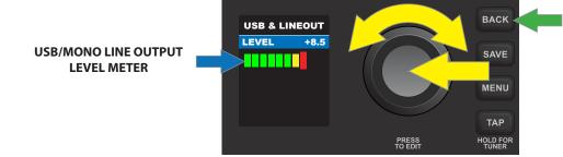
For best sound quality, set the "LEVEL" so that signal stays within the green bars, barely reaches the single yellow bar at right, and *does not* reach the single longer red clipping bar at far right (*all bars shown illuminat-ed in illustration above*). Note that changing presets can change individual volume; "LEVEL" readjustment may be necessary when changing presets.
