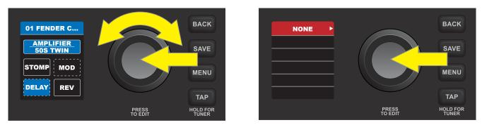
Turn the ENCODER *clockwise* to scroll through effects models in that category. Press the ENCODER on the desired effect, after which the box surrounding the effect name will return to blue and the effect is added—although not yet saved—to that effect category box. Alternately, press the BACK utility button (*green arrow*) to return to the preset contents screen (*see illustrations on next page*):
