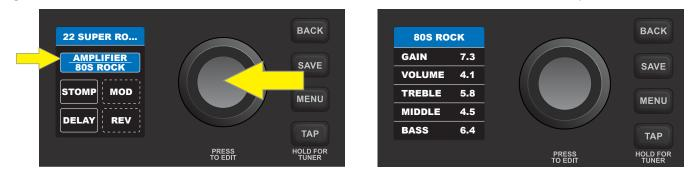
There are two ways to adjust an amp control knob setting. A control parameter that corresponds to an actual physical knob on the control panel can be adjusted simply by turning the physical control knob until the desired value is reached in the DISPLAY WINDOW. In the example below, the amp model's TREBLE setting is adjusted by turning the physical TREBLE control knob on the control panel:
