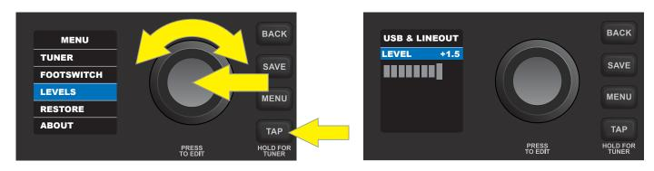
Turn the ENCODER to set a new "LEVEL" value. Press the ENCODER to accept the new value and exit the menu. Alternately, press the BACK utility button (*green arrow*) to accept the new value and return to the MENU function screen:
