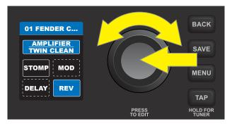
The DISPLAY WINDOW will then show a list of controls for the effect model in use in that category; use the EN-CODER to scroll to a particular effect control. Press the ENCODER to select the effect control; its surrounding box will turn from blue to red. Turn the ENCODER to set a new value for the selected control value:
