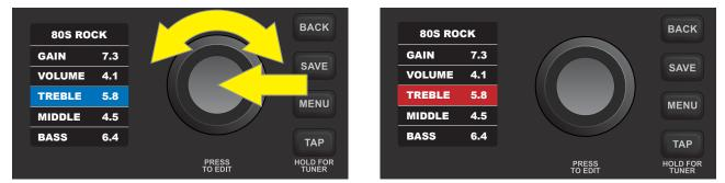
The control can then be adjusted by turning the ENCODER or by turning a corresponding physical control knob on the control panel:
