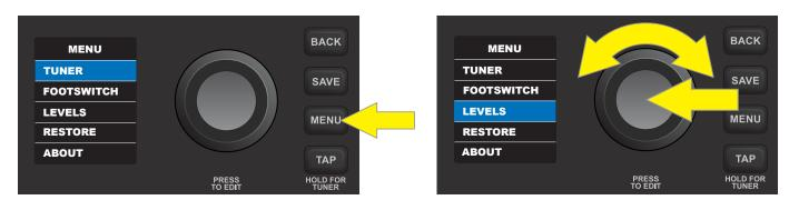
**TUNER:** Enables use of Mustang LT50's built-in chromatic tuner (*page 16*).
