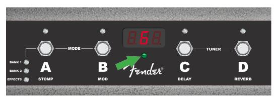
Here, the "G" note is at correct pitch, as indicated by the illumination of the green center LED (green arrow). When tuning is complete, step on any button to exit footswitch tuner mode.
