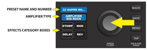
Select the amp model or one of the effects category boxes by turning and pressing the ENCODER. The active selection is then highlighted in blue:
