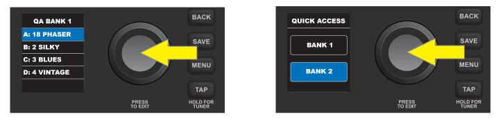
Once configured, all eight quick-access presets are easily accessible using the footswitch. When the amp is on and the footswitch is connected, BANK 1 is automatically active, and the four presets contained in it are assigned to footswitch buttons "A", "B", "C" and "D".
