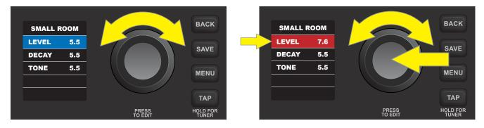
At this point, press the ENCODER to accept the adjusted effect control value and exit edit mode; the surrounding box will then return to blue. Alternately, press the BACK utility button (*green arrow*) to accept the effect control value change and return to the preset contents screen:
