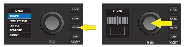
To use the TUNER, sound a note; the letter name of the pitch will appear in the box at bottom and the shorter vertical bars on either side of the longer vertical center bar will illuminate red to indicate varying degrees of sharpness (to the right) or flatness (to the left). When a pitch is precisely in tune, the longer vertical center bar and the two shorter vertical bars on either side of it will illuminate green:
