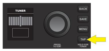
The second way is to press the MENU utility button on the control panel; the list of MENU functions will appear in the DISPLAY WINDOW with the TUNER function automatically highlighted atop the list. Press the ENCODER on TUNER to access the tuner screen:
