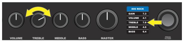
Alternately, select a control parameter by turning and pressing the ENCODER; its surrounding box will turn from blue to red:
