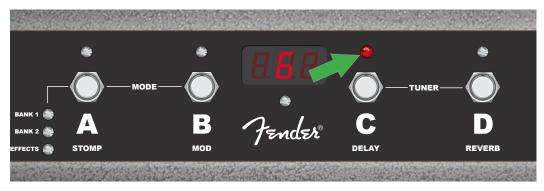
Here, the "G" note is displayed as slightly sharp, as indicated by the illumination of the red LED above button "C" (green arrow).
