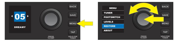
To initiate restoration use the ENCODER to scroll to and select "YES RESTORE". To cancel restoration, press the EN-CODER on "NO CANCEL", or press the BACK utility button. While restoration is in progress, a blue waiting screen with a progress bar will appear. When restoration is complete, the user is returned to the first preset screen:
