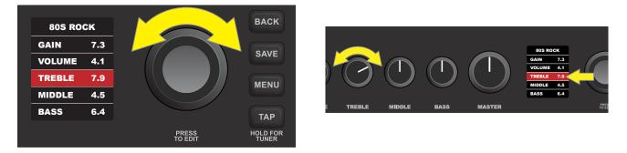
At this point, press the ENCODER or the BACK utility button (*green arrow*) to accept the adjusted control values. Pressing BACK returns the user to the preset contents screen; pressing the ENCODER lets the user continue making controls setting changes, and the box surrounding the control setting will return to blue. When control setting edits are complete, press the SAVE utility button to save the changes to the preset.
