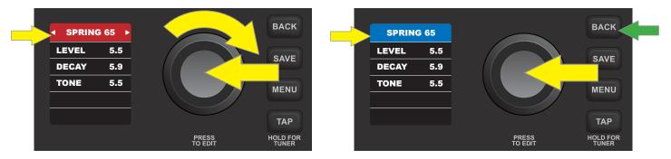
To **delete** an effect, the steps are very similar to those on page 10. As before, access the contents of a preset by pressing the ENCODER on it, then use the ENCODER to scroll to an occupied effect category box. Press the ENCODER again to see the effect contained in the effect category box; the name of the effect model is highlighted at the top of the DISPLAY WINDOW:
