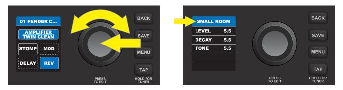
Press the ENCODER once more to activate the effect replacement function; the box surrounding the effect name will turn from blue to red, and white arrows will bracket the effect name. Turn the ENCODER *counter-lockwise* until the red-highlighted effect label at the top of the DISPLAY WINDOW reads "NONE". Press the ENCODER on "NONE" (or press the BACK utility button), after which the user is returned to the preset screen with the previously occupied effect category box now empty:
