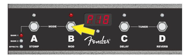
To access the presets in BANK 2, step on buttons "A" and "B" simultaneously. The green "BANK 2" LED at far left will illuminate, indicating that the four presets in BANK 2 have been assigned to footswitch buttons "A", "B", "C" and "D". As before, step on the button corresponding to the desired preset. In the example here, preset 5 has
