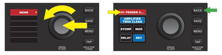
To **add** an effect to an empty effect category box, first access the contents of a preset by pressing the ENCODER on it, then use the ENCODER to scroll to the empty effect category box. Press the ENCODER again to access the empty effect category box; the red-highlighted label "NONE" will appear at the top of the DISPLAY WINDOW:
