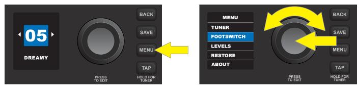
Both quick-access preset banks will appear in the DISPLAY WINDOW below the header "QUICK ACCESS"; the upper bank ("BANK 1") is automatically highlighted in blue. Press the ENCODER on it, and the four preset slots in the first bank appear with their default settings, labeled "A", "B", "C" and "D" to correspond to the "A", "B", "C" and "D" buttons on the footswitch. The first preset slot ("A") will be highlighted in blue:
