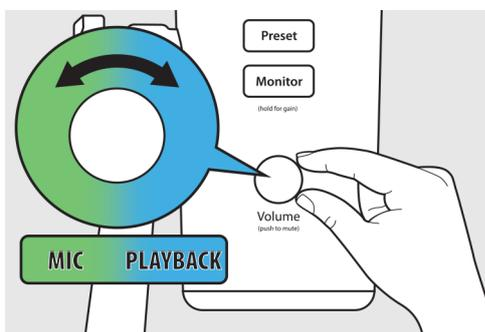
Turning the knob to the left will increase the level of the input signal relative to the playback from your computer. Turning it to the right will increase the level of the
