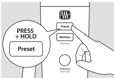
To bypass the presets, just press and hold the Preset button. The button will illuminate red while presets are bypassed.
