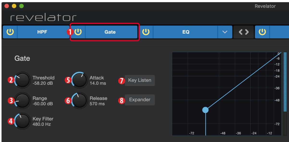
1. **On/Off.** Turns the Noise Gate on or off in the signal chain.
