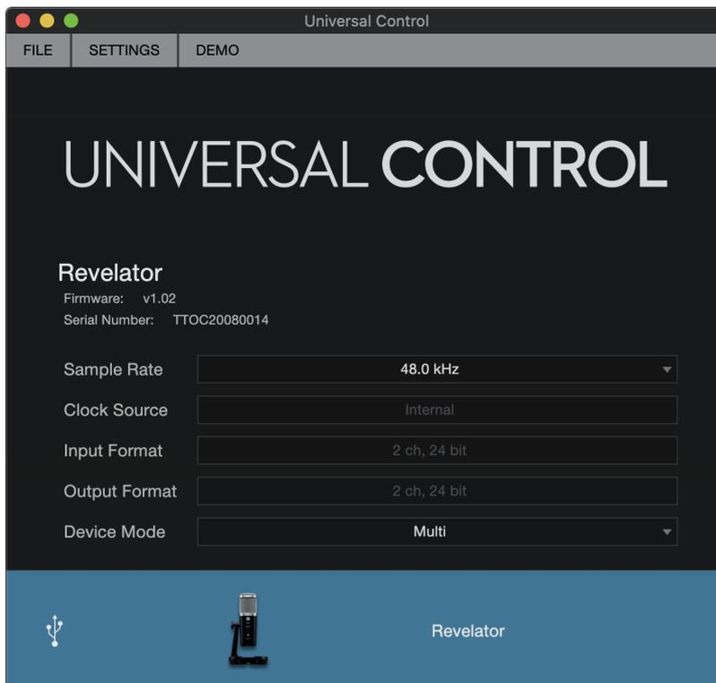
1. **Sample Rate.** Changes the sample rate. You can set the sample rate to 44.1, 48, 88.2, or 96 kHz. (With Multi Mode on macOS, the sample rate is limited to 44.1 and 48kHz.) A higher sample rate will increase the fidelity of the recording, but will also increase the file size and the amount of system resources necessary to process the audio.
