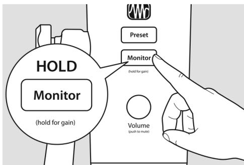
To set your Revelator's input level, press and hold the Monitor button. The Volume knob will turn green, letting you know that it is now controlling the microphone level.
