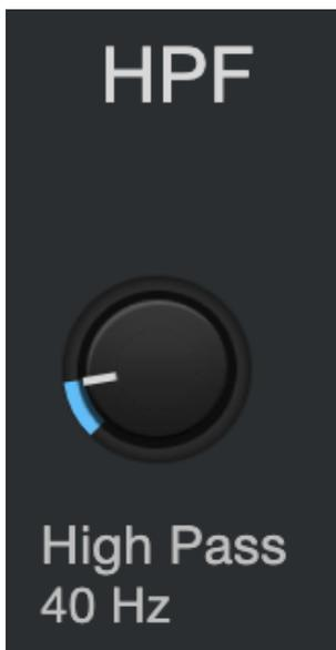
Use this control to set the High-Pass Filter frequency threshold for the selected Channel or Output Bus. The filter's threshold can be set from 24 Hz to 1 kHz. When the threshold is set to its lowest point, the filter is off. The high-pass filter's slope is -12 dB/8va.
