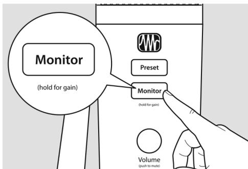
Press the Monitor button and turn the knob to adjust the blend between your microphone and the playback from your computer. The knob will be blue in this mode.
