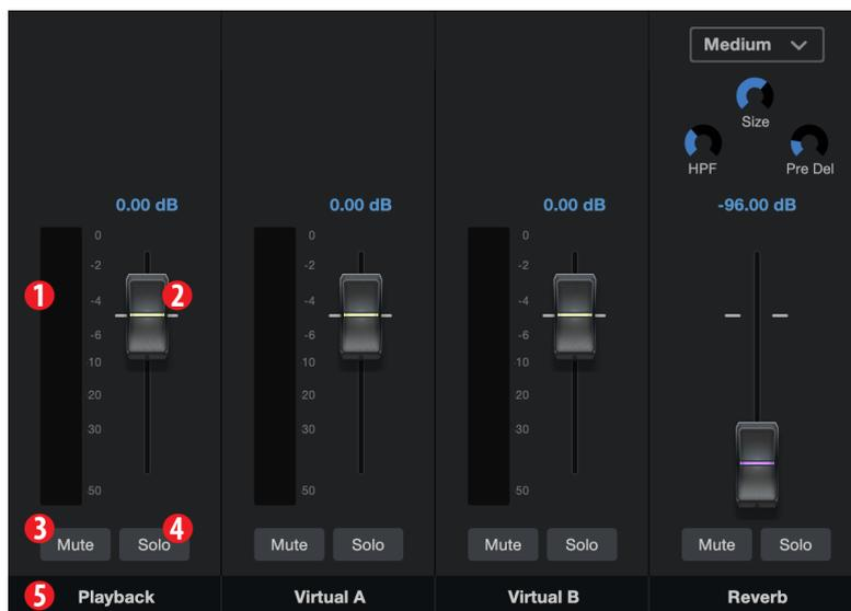
1. **Channel Meter.** This meter displays the current level of the channel before the fader (#2) level.
