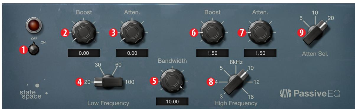
1. **On/Off.** Turns the EQ on or off in the signal chain.
