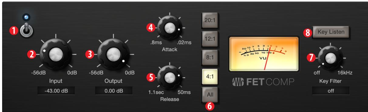
1. **On/Off.** Turns the Compressor on or off in the signal chain.
