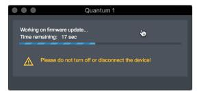
When the firmware update is complete, you must disconnect the physical power source from your Quantum-series interface and reconnect it. Powering it off it will not complete the update process.
