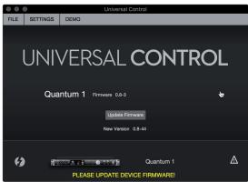
**Warning:** Do not power off or disconnect your Quantum-series interface during the firmware update. Once the firmware update is successfully completed, you will be alerted and instructed to disconnect your power supply and Thunderbolt cable and reconnect it before rebooting your device. *It is not sufficient to simply power down your unit, you must disconnect the power source.*
