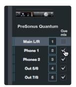
You can create a cue mix and send it to any output on your Quantum (Mains, Headphones, General Purpose, ADAT, or S/PDIF). You simply need to create an output bus and enable Cue Mix.
