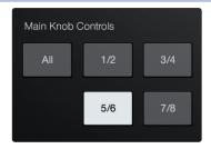
The large Main level encoder can be used to control any or every output on your Quantum-series interface. Use these controls to select which output levels are adjusted with this knob. It should be noted that this knob always controls the Main Left/Right outputs on Quantum and Outputs 1/2 on Quantum 2. Other analog outputs pairs can be added.
