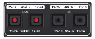
**ADAT – S/MUX In and Out.** These are the ADAT – Dual S/MUX connections for your external digital devices. When recording or playing back at 44.1 or 48 kHz, each ADAT I/O will provide 8 of the 16 available channels consecutively, from left to right. When recording or playing back at 88.2 or 96 kHz, each connection will provide four of the available eight channels.
