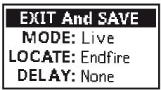
Your two AIR-series subwoofers will now radiate in a directional cardioid pattern, allowing you greater steering control over low-frequency energy with better off-axis rejection.
