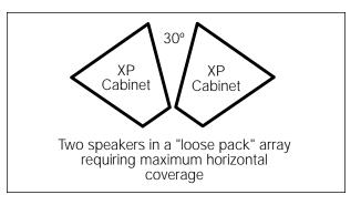
NOTE: When setting up your XP Series enclosures, be sure to place the cabinets in such a way as to minimize overlapping radiating patterns.
