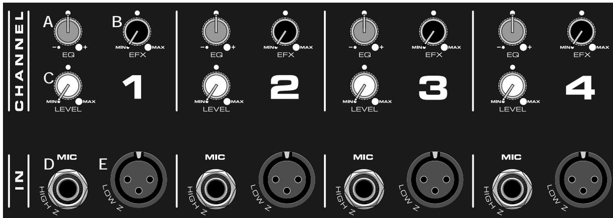
**A. EQ** - Adjusts the tone / frequency boost or cut of its respective channel. When the tone control is set at the 12 o'clock (notched) position, the channel is "flat" with no frequencies cut or boosted. As the dial is rotated clockwise, the treble response increases. Likewise, as the dial is rotated counterclockwise the treble response decreases.
