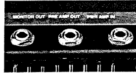
Preamp out/power amp input/patching facility.
