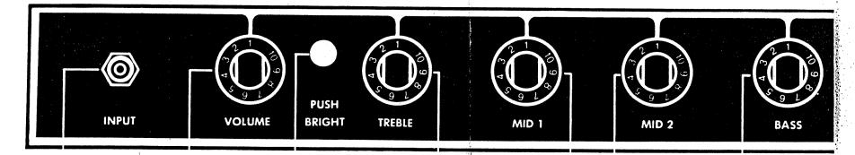
INPUT Connection for instrument VOLUME Volume setting from zero to full power PUSH BRIGHT Push Bright adds "brilliance" to the upper frequencies TREBLE Provides high frequency equalization as required MID 1 Provides upper midrange equalization (500 Hz 15 dB cut and boost)
