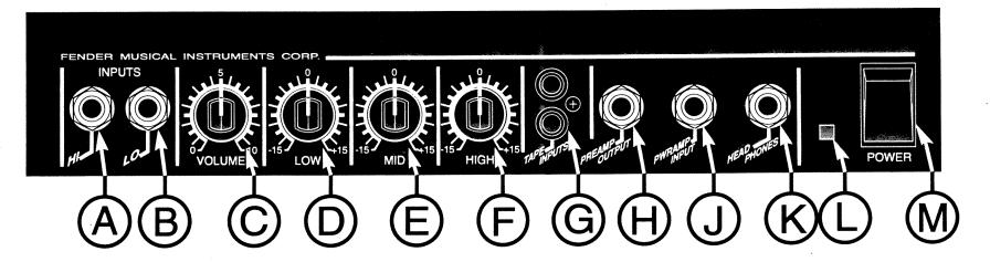
The front panel contains all items necessary for system operation and observation. Please read this section of the manual carefully to make sure you understand all the operational features of your new FENDER R.A.D. BASS amplifier.
