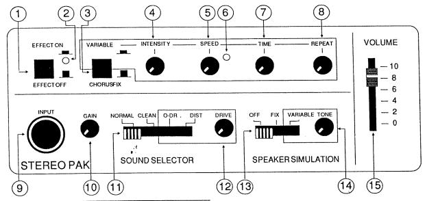
THE STEREO PAK is a portable stereo headphone amp incorporating best possible sounds and effects of use to every guitarist. Two or more players, each equipped with a STEREO PAK and a conventional stereo cable can play together, each hearing his own and the other player's sound simultaneously in full stereo. Rhythm machine or drum computer can be additionally added to these two signals and all three can be simultaneously recorded.
