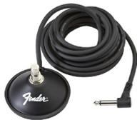
Connect a (optional) 1-button footswitch (P/N 0994049000) into the FTSW jack to enable remote selection of your two favorite presets. The LED (next to the FTSW jack) will turn **red** or **green** to indicate which footswitch preset is active.
