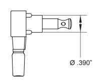
TUNING MACHINE THRU-HOLE INNER DIAMETER .397"
