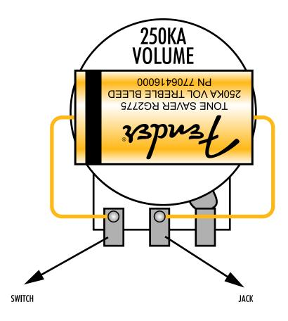
If you experience tonal change when turning down the volume control on your guitar, the **Fender Tone Saver**® is a great solution. Unlike traditional treble bleed circuits that involve connecting tiny parts together with delicate soldering, the **Tone Saver** contains a special R/C network inside one convenient enclosure that will keep your guitar's tone remarkably consistent at any setting. Just solder the leads to the center and outside lugs of your guitar's volume control and you're done.
