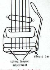
to the slot immediately above. Replace the Vibrato Unit to the body, string and tune to standard pitch. It may be once again necessary to adjust the spring tension at the two posts with the allen wrench.
