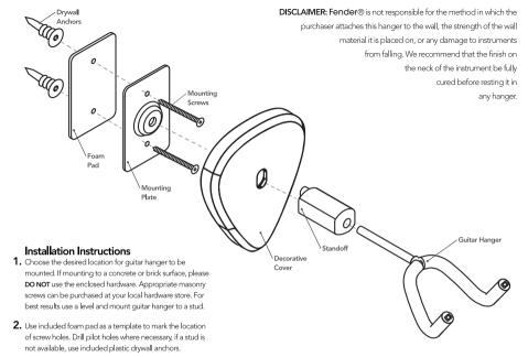
Attach foam pad to back of mounting plate and drive the supplied screws through the mounting plate into stud or plastic drywall anchors using a Phillips screwdriver.
