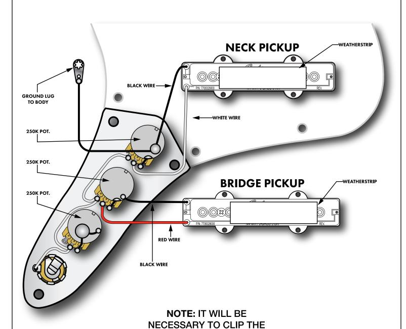
PCB PLUGS OFF IN ORDER TO INSTALL ON BASSES THAT DO NOT HAVE THIS FEATURE.
