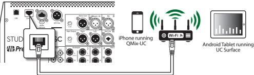
Ethernet cable from Control port to LAN connection on wireless router
