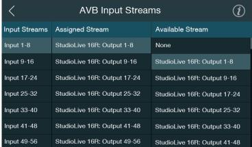
To change a routing, press the Input Stream to which you'd like to route and then use the value encoder to scroll through the Available Streams list on the right. Tap on the desired routing to patch it.
