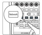
If you would like the input source for any channel on your StudioLive Series III console mixer to come from your StudioLive Series III rack mixer, select that channel on your console mixer and enable Network as the Input Source. For example, if you would like to use the guitar connected to Input 3 on your StudioLive 16R in any mix on your StudioLive 32S, you would select Channel 3 on your StudioLive 32S and enable Network as the input source.
