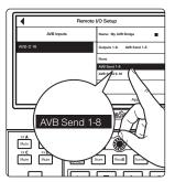
6. Select the drop down menu for Outputs 1-8 to choose an AVB stream to send to the AVB-D 16. Note that you must have a stream connected here to ensure the AVB-D 16 is receiving a proper media clock. Repeat for channels 9-16.
