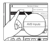
7. Select the AVB Inputs button at the top left of the touch screen to route audio from the AVB-D 16 to the StudioLive Series III mixer.
