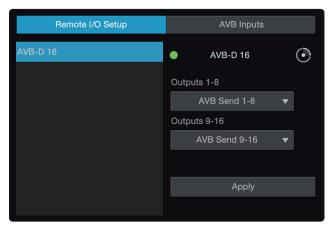
4. With the AVB-D 16 selected you'll see the setting options on the right hand side of the Remote I/O Setup area.
