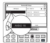
4. On the Remote I/O Setup screen you will see the AVB-D 16 in the list of devices on the left hand side of the screen. If you have any NSB-series stage boxes, EarMix 16M or other StudioLive Series III mixers connected to the same AVB network, you will also see them in the list. Select the AVB-D 16. Once the AVB-D 16 is selected, you'll see the setting options on the right hand side of the touch screen.
