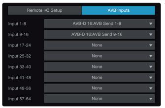
7. Select the AVB Inputs tab at the top of this area to route audio from the AVB-D 16 to the StudioLive Series III mixer. On the AVB Inputs screen select an incoming stream from the list of the left hand side of the screen. Choose an available AVB stream from the list on the right to route that stream to the input currently selected on the left. If you don't see the stream on the right you may need to scroll further down the list.
