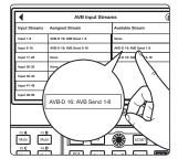
8. On the AVB Inputs screen select an incoming stream from the list of the left hand side of the screen. Choose an available AVB stream from the list on the right to route that stream to the input currently selected on the left. If you don't see the stream on the right you may need to scroll further down the list using the encoder in the master control area of the mixer.
